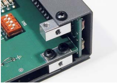
Figure 45. Attaching 2-D Fasteners to Cabinet End Covers.
