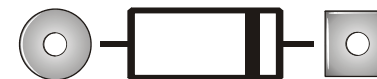
Figure 16. PCB Diode Orientation Guides. The cathode always goes to the square solder pad on the PCB.
