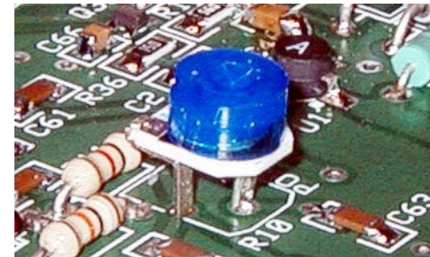
Figure 18. Installing R10. Orient the center pin toward the beveled end of the silk-screened outline.
