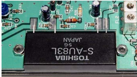
Figure 40. RF PCB attached to the RF Power Module Screws.
