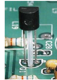
Figure 23. Installing Q1 with Teflon Spacer.
