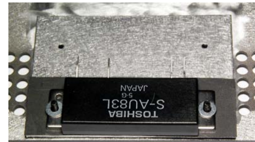
Figure 39. RF Power Module and Flat Washers in Place on the Heat Spreader.
